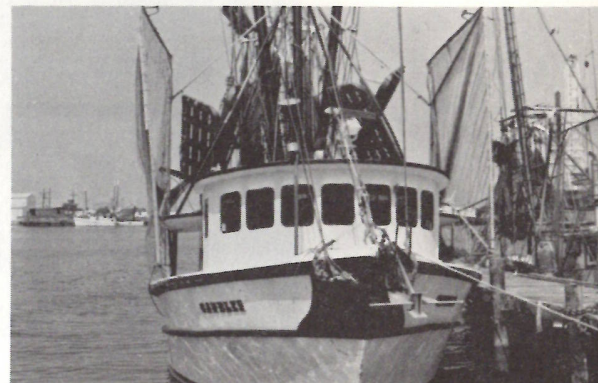
Large shrimp boat rigged for both "butterfly" and trawl fishing.
