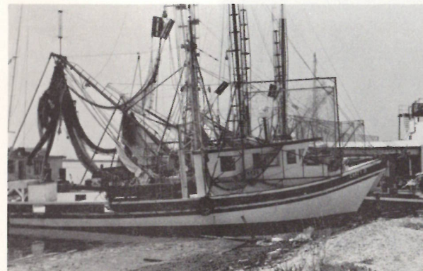
Typical commercial "butterfly" rigged shrimp boat. Conventional trawl shrimp gear can also be used as can be seen above back deck.
