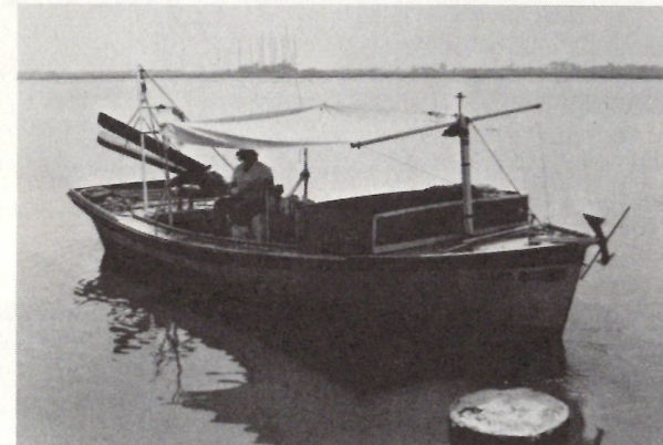
Inland "skiff" type shrimp boat used in inland waters and along the Cameron Parish beaches.
